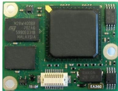
**Figure 1-2 Jupiter Pico T GPS receiver (bottom view)**
